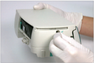
Turn crank inside aperture to open the door.
