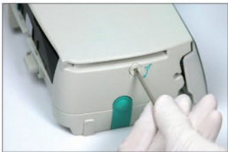
Turn crank to remove emergency aperture cover.
