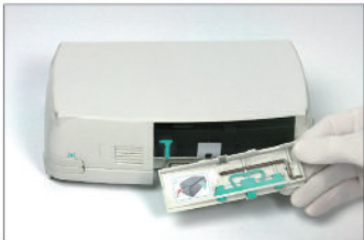
Remove crank from inside of battery cover.
